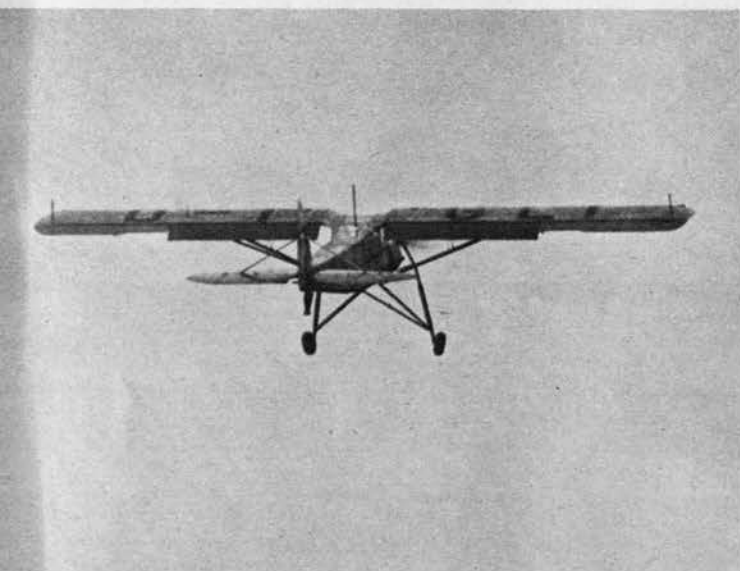
The Fieseler-156 , which is known as the Storch (Stork) because of long-legged fixed landing gear, is principal Luftwaffe liaison type. This light, insect-like airplane is somewhat faster than our L series.
